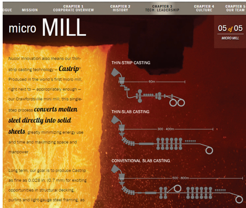
Fig. 7. Length difference between Nucor thin-strip casting and conventional slab casting, http://www.nucor.com/
