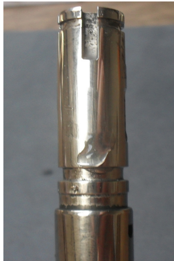
Fig. 2. Water drop on chemical nickel coating at one piston from fuel engine, photographed in vertical position of the piston
